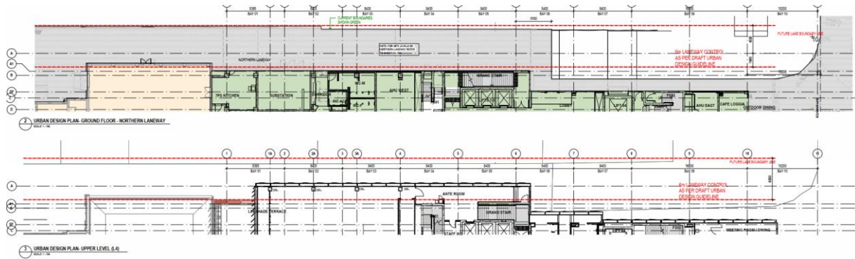
Figure 18: Northern laneway alignment at ground and upper level with overhang (Source: extract of DA-1610)
